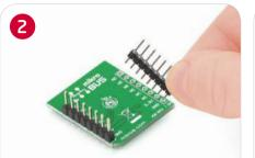
Turn the board upside down so that bottom side is facing you upwards. Place shorter pins of the header into the appropriate soldering pads.
