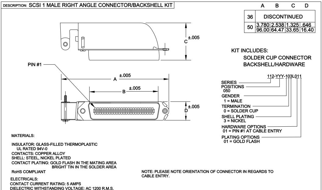
INSULATION RESISTANCE: 1000 mohms MINIMUM AT 500V DC
