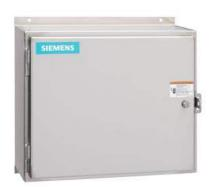
Mechanically held lighting contactor, Contactor amp rating 60Amp 0NC  $\_$  8NO poles, 277VAC 60HZ coil, Non-combination type, Enclosure NEMA type 12, Dust/drip proof for indoors
