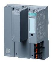
SCALANCE XF204-2BA DNA managed IE Y-switch, IEC 62443-4-2 certified; 4 x 10/100 Mbit/s, 2 x BusAdapter interface, error signaling contact, set pushbutton, redundant 24 V DC power supply, PROFINET device, extended temperature range -40  $^{\circ}$ C...+70  $^{\circ}$ C, conformal coating, with electr. manual on DVD, C-PLUG optional, supplied without BusAdapter
