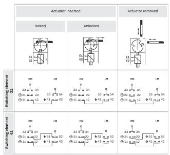
$<sup>\</sup>frac{1}{\mathbf{k}^{\prime}}$  Positive action N/C locking monitoring contact
