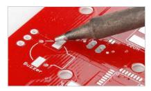
Pre-tin the start-pad by feeding solder into the joint.
