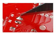
B Using a soldering iron, close both jumpers.
