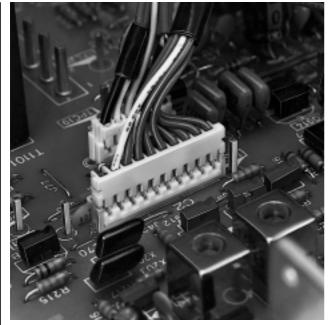
This 2.5mm (.098") pitch connector for printed circuit boards has an ultra-thin construction. The in-line method provides high-density capability to the end user.
