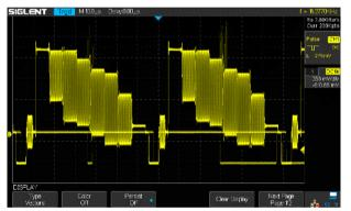
256-level intensity grading display on waveform
