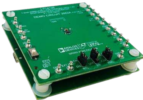
Figure 7. DC2662A mounted on top of DC2661A
