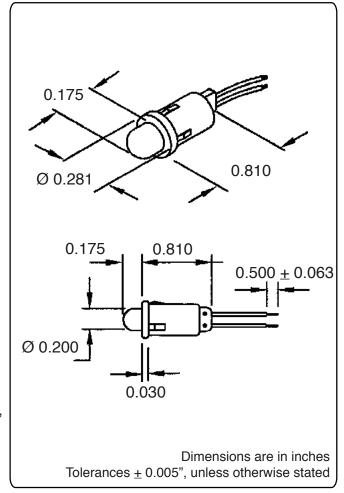
LED Indicator Light 2 to 24 Volts DC Clear or Diffused LED 1/4" Mounting Hole
