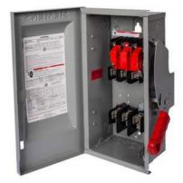
Siemens Low Voltage Circuit Protection Heavy Duty Safety Switch. 3-Pole 3-Wire and negative ground Non-Fused in a type 3R enclosure (outdoor). Rated 600VAC (200A). Special features: photovoltaic rated, 10000 AIC disconnect.
