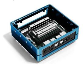
**Stackable structure to extend endless possibilities for building different applications such as NAS.** If your application requires more space, for example, adding more hard disks to make a NAS, the stackable structure allows you to stack more middle layers to create rooms very easily.
