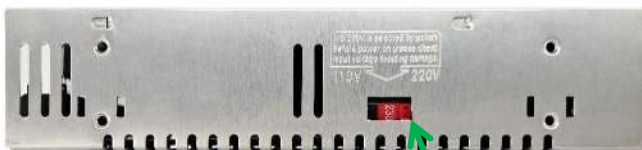
220VAC Input Voltage
