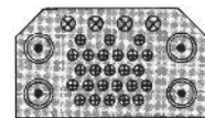
Arrangement 33C4 25 Size 20 contacts 4 Size 16 contacts 4 Size 15 COAXICON contacts, 4 Size 5 COAXICON contacts
