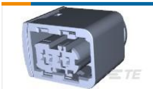
TE Part #3-1418483-1 2POS,AMP MCP2.8,REC. HSG
