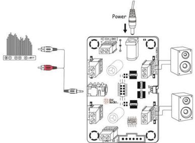
The gain on this amplifier board is fixed at 26 dB. Please use your audio source device's volume control to adjust the amplifier output. Alternatively, you can connect a 25 kOhm audio taper potentiometer between the audio source device and amplifier for the purpose of volume control.
