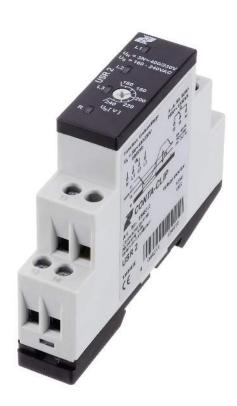
Undervoltage monitoring relay module with adjustable switching threshold (160 - 240 V), Screw connection, Mounting type: Mounting rail TS 35, 1 CO contact
