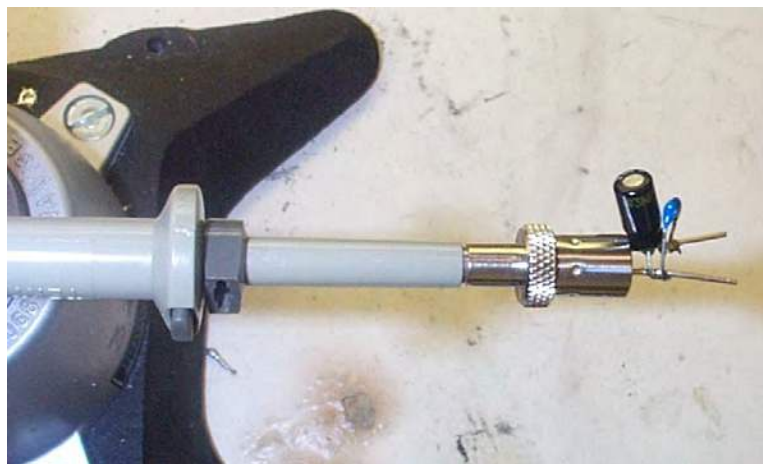
Figure 47 – Oscilloscope Probe with Probe Master 4987BA BNC Adapter (Modified with Wires for Probe Ground for Ripple measurement and Two Parallel Decoupling Capacitors Added).
