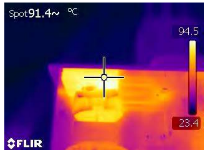
Figure 52 – Input Rectifier Bridge (BR1), 90 VAC Input, 100% Load, Room Temperature.
