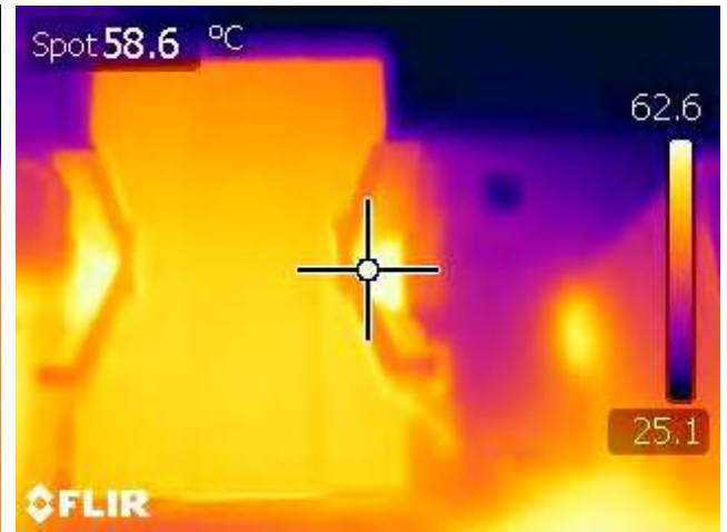
Figure 64 – PFC Inductor (L2), 115 VAC Input, 100% Load, Room Temperature
