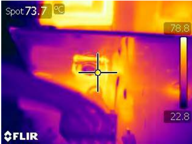
Figure 57 – Output Rectifier (D11), 90 VAC Input, 100% Load, Room Temperature.
