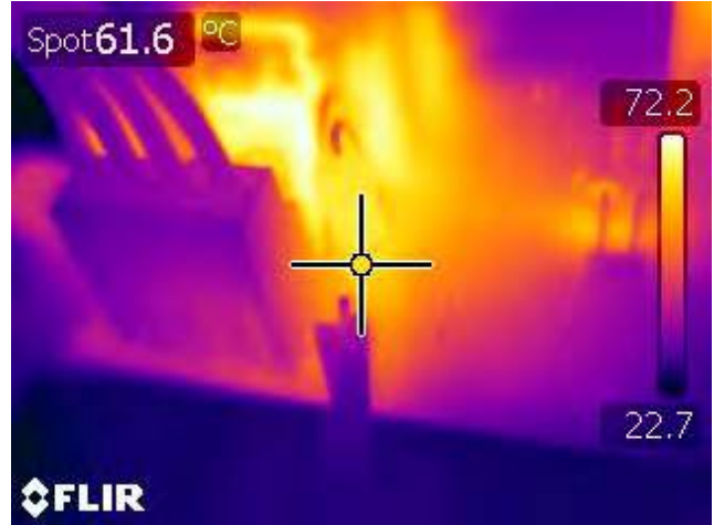
Figure 68 – Current Sense Resistor (R53), 115 VAC Input, 100% Load, Room Temperature.
