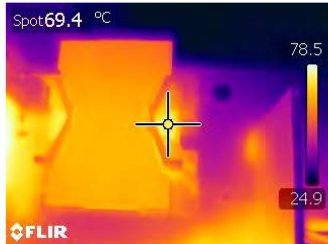
Figure 54 – PFC Inductor (L2), 90 VAC Input, 100% Load, Room Temperature.
