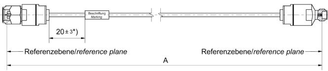
All dimensions are in mm; tolerances:  $\pm$  3mm for A  $\leq$  300 mm;  $\pm$  1% for A > 300 mm \*) If length "A"  $\leq$  90 mm marking is mount centric  $\pm$  5mm
