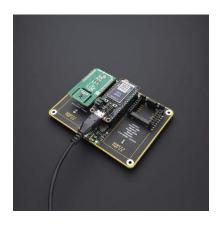
When USB mini connector is connected to the Feather base-board the PWR diode will glows Green, at this setup the Feather base board itself will be powered and will provide power to the shield including two mikroBUS sockets. The maximum current that Feather main board can provide over USB cannot exceed 500mA.
