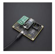
When USB type C connector is connected to the shield the PWR diode will glows Blue, at this setup the connected Feather base-board and two mikroBUS sockets will be powered from it. Maximum overload on the mikroBUS connectors should not exceed 2A on 3.3V, and load on 5V will depends directly from the current that can supply USB source to which this shield is connected (PC, USB hub, etc).
