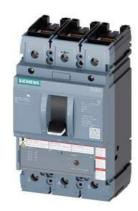
circuit breaker 3VA5 UL frame 250 3-pole, starter protection TM120M, AM, In=200A without overload protection short-circuit protection Ii=6...12 x In cable connection on both sides
