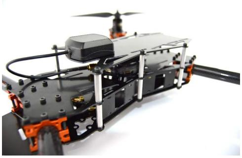
The frame is compatible with the <u>Lynxmotion Quadrino Nano Flight Controller</u> (not included) with a section designed for the GPS antenna and access to the underside ports. There are integrated mounting plates for the ESCs which allow for easy access.
