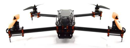
We equipped the HQuad500 with a camera plate up front which is removable. Different plates will be available as well as a stabilized gimbal system. The flight controller mounting is located at the "dead center" of the frame with slots accommodating 30.5mm to 45mm mounting.
