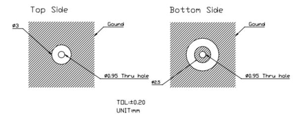
\*Note Layout Dimensions may be affected by the thickness of the PCB
