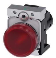
Indicator lights, compact, 22 mm, round, metal, red, lens, smooth, with holder, Operating voltage 24 V AC/DC, screw terminal
