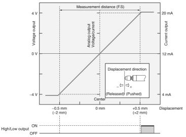
Note: To prevent destroying the Sensor Head, both the high and low judgment outputs will light if 101% of the upper limit of the measurement distance is reached.
