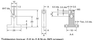
Tightening torque: 0.6 to 0.8 N·m (M3 screws) Material: Aluminum
