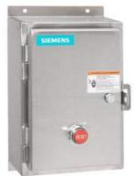
Non-reversing motor starter, Size 1, Three phase full voltage, Solid-state overload relay, OLR amp range 0.75-3.4A, 24VAC 50-60Hz coil, Non-combination type, Encl. type 4X 304 S. Steel, Water/dust tight noncorrosive, Standard width enclosure
