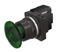
30mm BlackMax, Epoxy Coated Corrosion Resistant Metal Operator, Round Illuminated Twist-to-Release Transformer type, 240V AC LED Lamp Mushroom Head Cap Small 1.79" (45 mm) Plastic Cap, Green 2 Position Maintained, Twist-to-Release UL Listed, CSA Certified NEMA 1,3,3R,4,4X,12,13 & Automotive Standards
