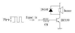
Resonant frequency, 1/2 duty cycle. Square wave. Signal amplitude should be large enough tosaturate the transistor.
