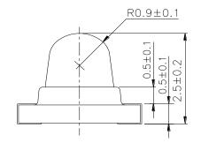
For reflow soldering (propose)
