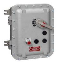
Non-reversing motor starter, Size 1 3/4, Three phase full voltage, Solid-state overload relay, OLRelay amp range 10-40a, 110V 50HZ / 120V 60HZ coil, Combination type, 60Amp fusible disconnect, 60Amp / 600V fuse clip Encl. NEMA type 4X Fiberglass Water/dust tight noncorrosive, Standard width enclosure
