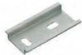
TS 35/7.5 mm according to EN 50022 (s = 1.0 mm)
