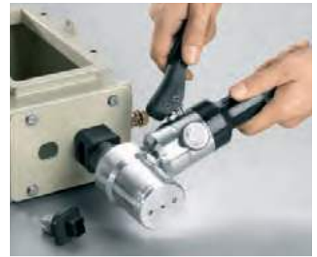
Punching out holes for a variety of industrial Ethernet connectors.
