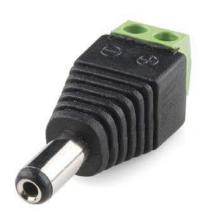
**Description:** This adapter allows you to connect a barrel jack connector to bare wires. One end has screw terminals and the other has a 5.5x2.1mm, center-positive male barrel jack. If you need to connect bare wires to a barrel jack on an Arduino or a development board, this might be the simple solution.
