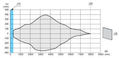
(X): Target distance (Y): Detection limit
