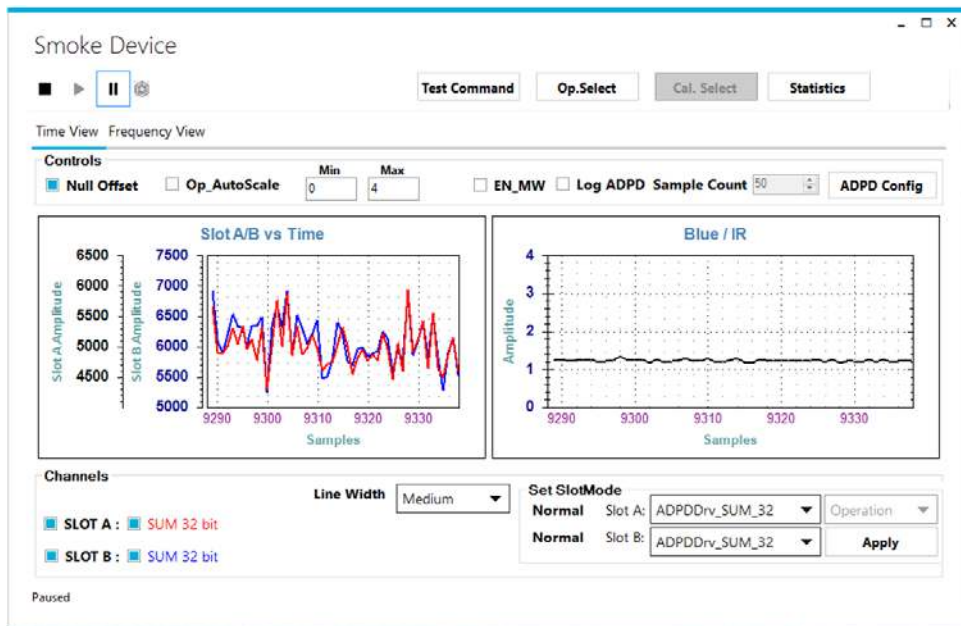
Figure 19. Raw Data Response and Blue/IR Ratio Measurement of Smoke Spray
