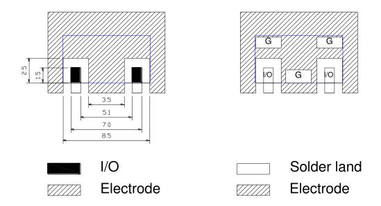
Shielding case layout guide (MIN)
