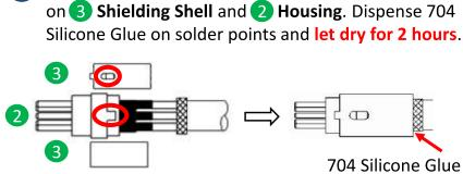
Assemble 3 Shielding Shells by matching the keying
