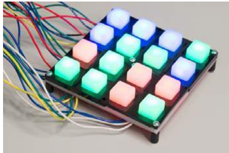
4x4 Button Pad with Arduino Mega 2560
