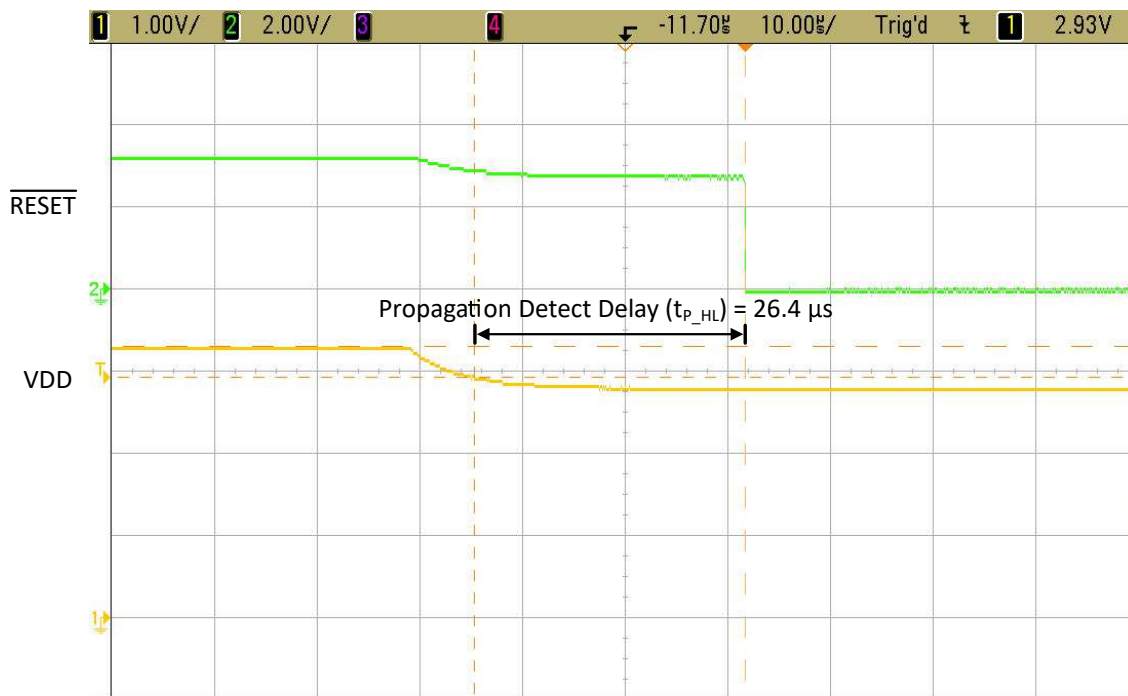
Figure 4-2. TLV841EVM \overline{RESET} Propagation Detect Delay
