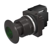
30mm BlackMax, Epoxy Coated Corrosion Resistant Complete Metal Unit Illuminated Push-Pull Operator Transformer type, 240V AC LED Lamp Mushroom Head Cap Small 1 3/4" (44.5 mm) Metal, Black with Green Lens 2 Position Maintained, Pull-to-Release UL Listed, CSA Certified NEMA 1,3,3R,4,4X,12,13 & Automotive Standards
