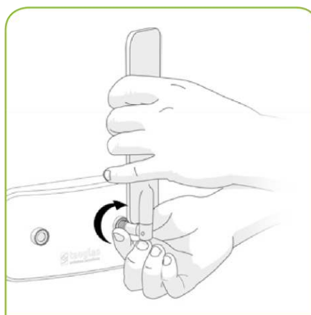
Figure 2. Fix the connector to the device by twisting the rotating head of the SMA connector until it is tight enough to hold the antenna in the correct position.
