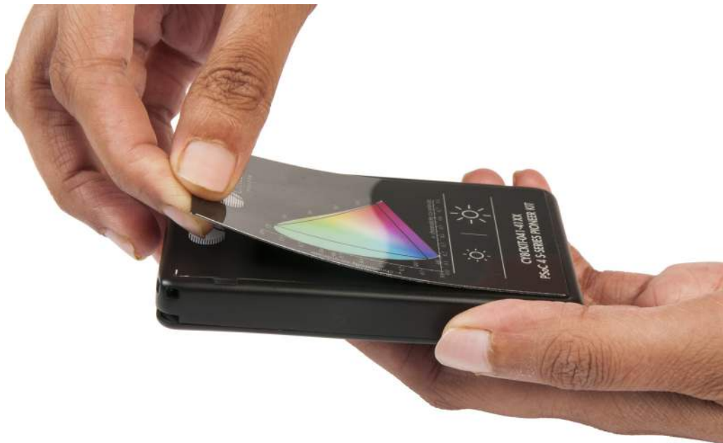
Figure 3-10. Removing the Overlay
