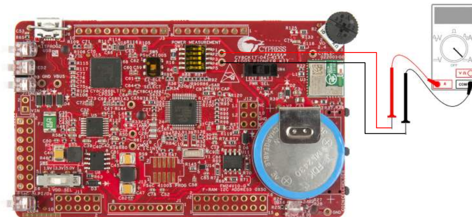
Figure A-6. Current Measurement when Powered from USB Connector or Battery
