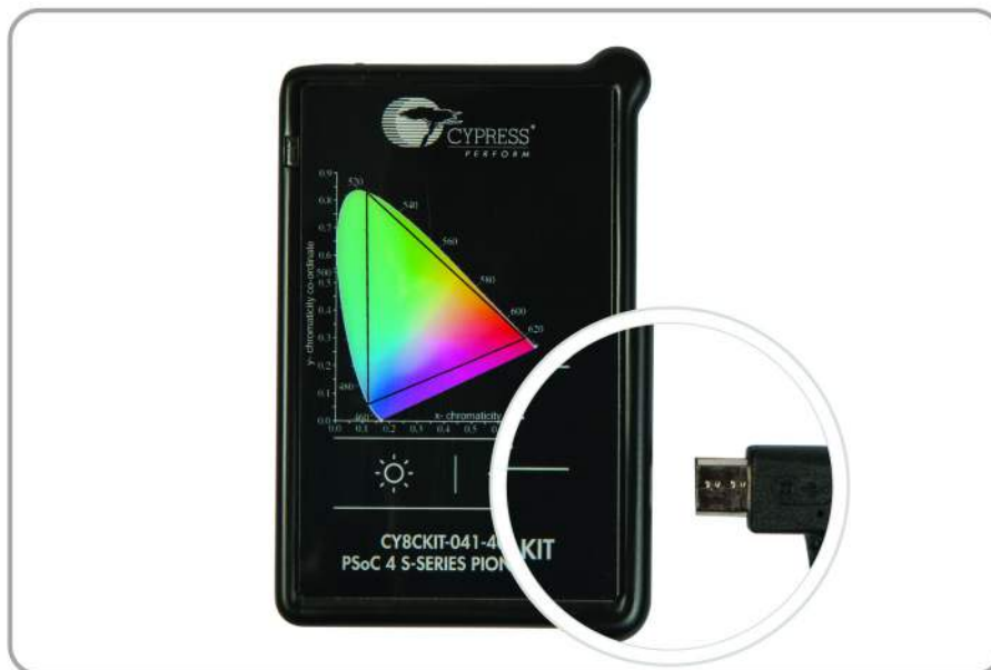
Figure 3-12. Connect USB Cable to USB Connector on the Kit
