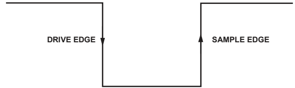
Figure 45. SPI Mode 3 SCLK Edges
