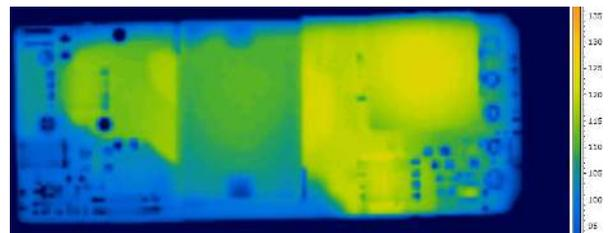
Figure 6. Thermal Image of CPE4D36 (4A output, 55C Ambient, 100lfm airflow, Vin = 48V, airflow from pin 3 to pin 1, Tmax = 122°C)
