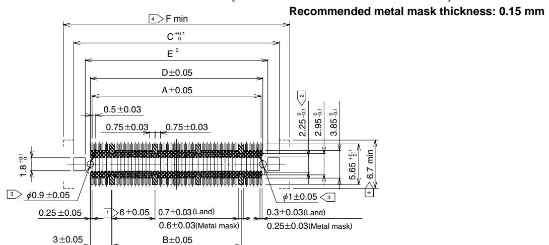
Note ① Cross-hatched portions, totaling n places, indicate the ground circuits.
