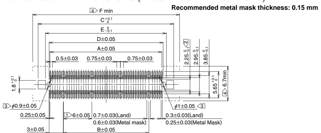
Note ① Cross-hatched portions, totaling n places, indicate the ground circuits.
