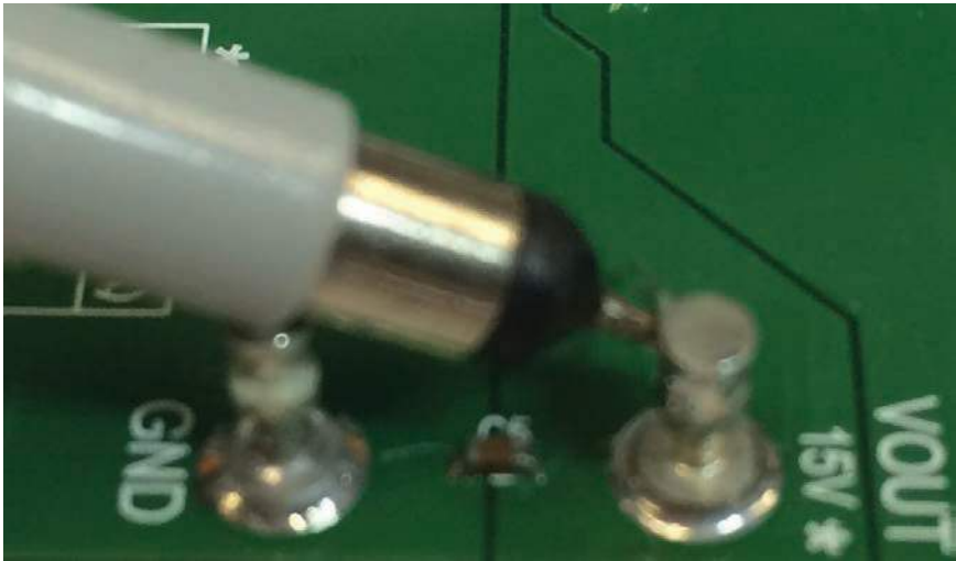
Figure 3. Output Ripple Measurement Technique
