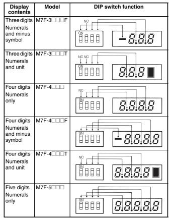
**Note: 1.** The minus symbol and decimal point are always lit when the corresponding pins of the DIP switch are set to ON.
