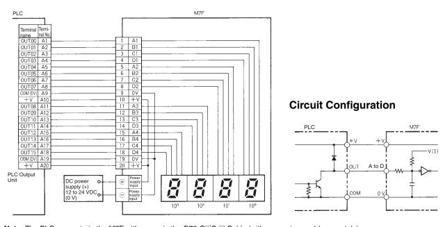
Note: The PLC connects to the M7F with ease via the G79-O C- Cable (with connectors, sold separately). (The above example indicates 1 to 1 connection.)
