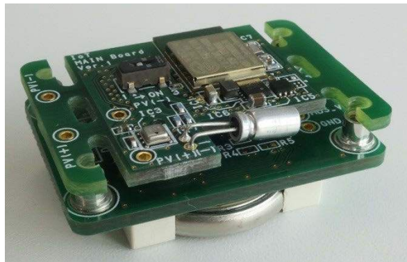
Picture: Connection with the RIOT-001 (The lower board is the RIOT-C01.)
