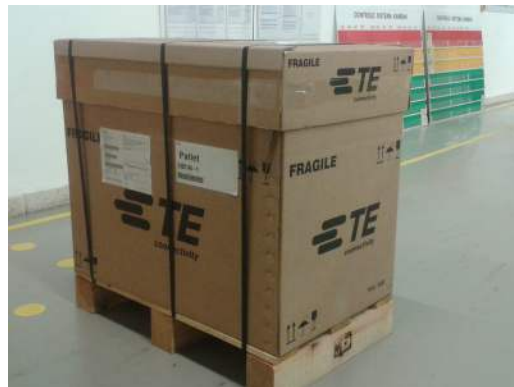
Fig. 1: Proper packing of relays for transportation
