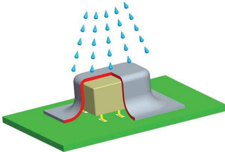
Fig. 4: Coating of relays on PCB's
