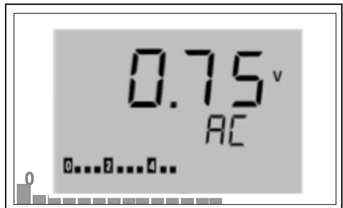
Figure 9. AC voltage display
