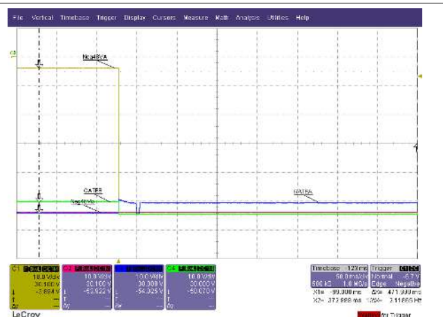
VinA = 54.5 V; VinB = 54 V, Scope GND = RTN, No load
